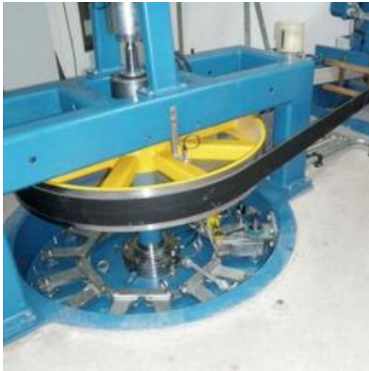
Figure 53: Flat belt drives in micro hydropower installations (Burger Wasserkraftanlagen, 2020)
