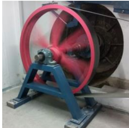
Figure 53: Flat belt drives in micro hydropower installations (Burger Wasserkraftanlagen, 2020)
