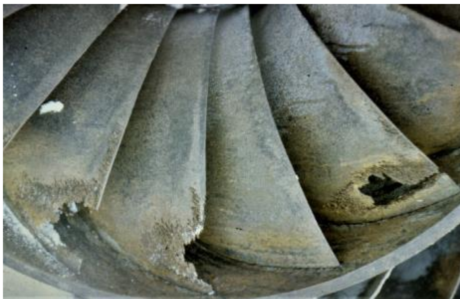
Figure 13: Extensive cavitation damage at the suction side of a small Francis turbine runner (1970s, source: IMP PAN archives)
